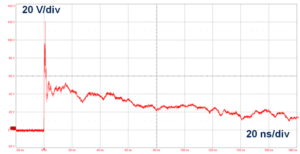
Figure 9. Response to ISO 10605 - C = 150 pF, R = 330 Ω (+8 kV contact )
