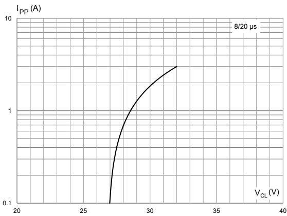
Figure 4. Peak pulse current versus clamping voltage (8/20 \mu s exponential waveform)
