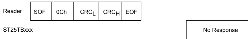
Figure 52. Reset_to_inventory frame exchange between reader and ST25TB04K
