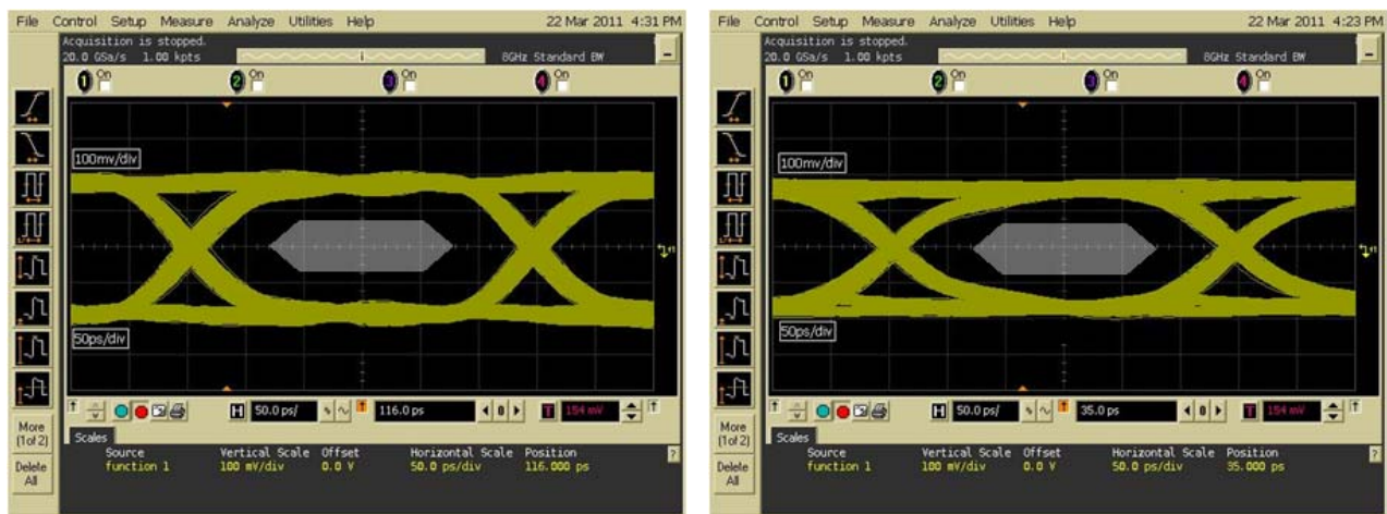
Figure 10. EMI4183 Measured Eye Diagram @ 3.4Gbps (EVB through on left, EVB with EMI4183 on right)
