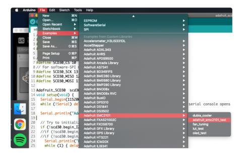
After opening the demo file, upload to your Arduino wired up to the EMC2101. Once you upload the code, you will see the Internal and External Temperature, Fan speed
