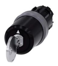
Key-operated switch BKS, 22 mm, round, plastic with metal front ring, lock number S1, with 2 keys, 3 switch positions I>O<II, momentary contact type, actuating angle 2x45°, 10:30h/12h/13:30h, key removal O, with laser labeling, lower case
