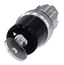
key-operated switch Siemens, 22 mm, round, metal, shiny, special lock, with 2 keys, 2 switch positions O<I, momentary contact type, actuating angle  $45^\circ,\,10:30h/12h,$  key removal O
