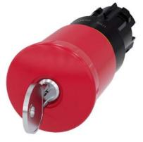
EMERGENCY STOP mushroom pushbutton, 22 mm, round, plastic, red, 40 mm, with lock Siemens, lock no. SSP9, positive latching, according to DIN EN ISO 13850, key-operated release Z=50-unit packaging
