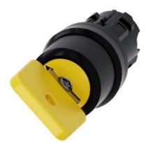
Key-operated switch O.M.R, 22 mm, round, plastic, lock number 73033, yellow, with 2 keys, 2 switch positions O<I, momentary contact type, Actuating angle 45°, 10:30h/12h, key removal O, with laser labeling, lower case
