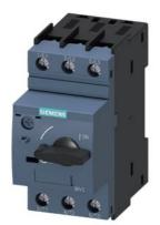
Circuit breaker size S0 for transformer protection A-release 18...25 A N-release 400 A screw terminal Standard switching capacity
