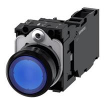
Illuminated pushbutton, 22 mm, round, plastic, blue, pushbutton, flat, momentary contact type, with holder, 1 NO+1 NC, LED module with integrated LED 24 V AC/DC, screw terminal, with laser labeling, upper case and lower case, Always upper case at the beginning of the word
