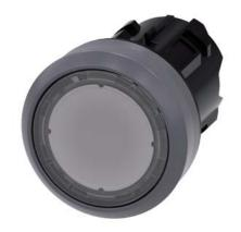
Pushbutton, 22 mm, round, plastic with metal front ring, clear, pushbutton, flat momentary contact type, with laser labeling, symbol number according to, ISO 7000 or IEC 60417
