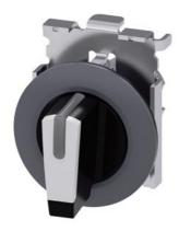
Selector switch, illuminable, 30 mm, round, Metal, matte, white, selector switch, short, front ring for flush installation, 3 switch positions I>O<II, momentary contact type, actuating angle 2x45°, 10:30h/12h/13:30h, with laser labeling, upper case and lower case, always upper case at the beginning of the word
