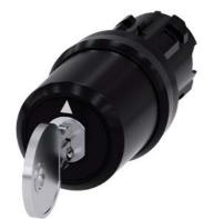
Key-operated switch BKS, 22 mm, round, plastic, Lock No. E2 (VW), without key, 3 switch positions I-O-II, latching, actuating angle 2x45°, 10:30h/12h/13:30h, Key removal I+O+II Z=50-unit packaging
