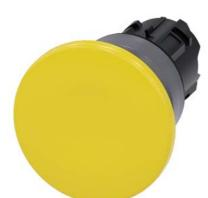
Mushroom pushbutton, 22 mm, round, plastic with metal front ring, yellow, 40mm, momentary contact type, with laser labeling, upper case
