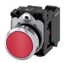
Pushbutton, 22 mm, round, metal, shiny, red, pushbutton, flat, momentary contact type, with holder, 1 NC, spring-type terminal, with laser labeling, upper case
