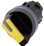
Selector switch, illuminable, 22 mm, round, plastic with metal front ring, yellow, selector switch, short, 2 switch positions O-I, latching, actuating angle 90°, 10:30h/13:30h, with laser labeling, inscription or symbol Customer-specific selection with SIRIUS ACT configurator (CIN)
