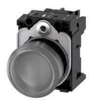
Indicator lights, 22 mm, round, plastic, clear, lens, smooth, with holder, LED module, with integrated LED 230 V AC, screw terminal, with laser labeling, upper case
