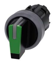
Selector switch, illuminable, 22 mm, round, plastic with metal front ring, green, selector switch, short, 3 switch positions I>O<II, momentary contact on the left, latching on the right, actuating angle 2x45°, 10:30h/12h/13:30h, with laser labeling, upper case and lower case, always upper case at the beginning of the word
