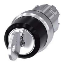
RONIS key-operated switch, 22 mm, round, metal, shiny, lock number SB30, with 2 keys, 3 switch positions I-O<II, left latching, right momentary contact type, actuating angle 2x45°, 10:30h/12h/13:30h, key removal I, possible special locks: SB31, 421, 455, with laser labeling, inscription or symbol Customer-specific selection with SIRIUS ACT configurator (CIN)
