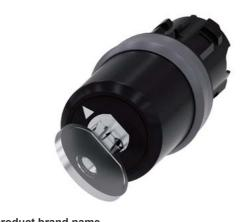
Key-operated switch BKS, 22 mm, round, plastic with metal front ring, lock number S1, with 2 keys, 2 switch positions O-I, latching, actuating angle 90°, 10:30h/13:30h, key removal I, with laser labeling, upper case and lower case, always upper case at the beginning of the word
