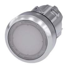
Illuminated pushbutton, 22 mm, round, metal, shiny, white, pushbutton, flat, latching, Push-to-release mechanism, with laser labeling, upper case and lower case, Always upper case at the beginning of the word
