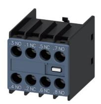
Auxiliary switch 11 U, on the front, 2 NO + 2 NC Current path 1 NO, 1 NC, 1 NC, 1 NO for 3RH and 3RT screw terminal .3/.4, .1/.2, .5/.6, .7/.8
