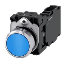
Pushbutton, 22 mm, round, metal, shiny, blue, pushbutton, flat, momentary contact type, 1 NO+1 NC, screw terminal, with laser labeling, symbol number according to, ISO 7000 or IEC 60417
