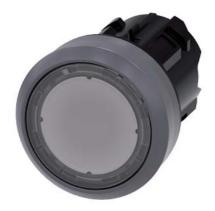
Pushbutton, 22 mm, round, plastic with metal front ring, clear, pushbutton, flat momentary contact type, with laser labeling, upper case and lower case, always upper case at the beginning of the word
