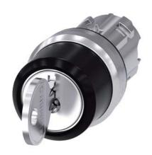
RONIS key-operated switch, 22 mm, round, metal, shiny, lock number SB30, with 2 keys, 3 switch positions I-O-II, latching, actuating angle 2x45°, 10:30h/12h/13:30h, key removal O, possible special locks: SB31, 421, 455, with laser labeling, upper case and lower case, always upper case at beginning of line
