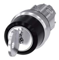
RONIS key-operated switch, 22 mm, round, metal, shiny, lock number SB30, with 2 keys, 3 switch positions I>O<II, momentary contact type, actuating angle 2x45°, 10:30h/12h/13:30h, key removal O, possible special locks: SB31, 421, 455, with laser labeling, lower case
