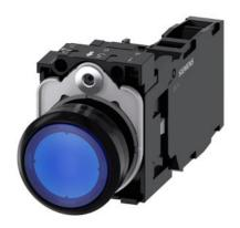
Illuminated pushbutton, 22 mm, round, plastic, blue, pushbutton, flat, momentary contact type, with holder, 1 NO+1 NC, LED module with integrated LED 24 V AC/DC, screw terminal, Z=20-unit packaging
