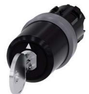
key-operated switch Siemens, 22 mm, round, plastic with metal front ring, lock number SSG10, with 2 keys, 3 switch positions I-O<II, left latching, momentary contact type on the right, actuating angle 2x45°, 10:30h/12h/13:30h, key removal O+I, with laser labeling, upper case
