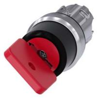
Key-operated switch O.M.R, 22 mm, round, metal, shiny, lock number 73037, red, with 2 keys, 2 switch positions O-I, latching, actuating angle  $90^{\circ}$ , 10:30h/13:30h, key removal I, with laser labeling, lower case
