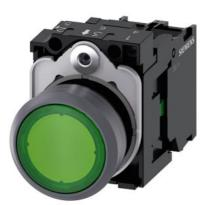
Illuminated pushbutton, 22 mm, round, plastic with metal front ring, green, pushbutton, flat, momentary contact type, with holder, 1NO, LED module with integrated LED 24 V AC/DC, screw terminal, with laser labeling, upper case
