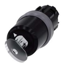
key-operated switch Siemens, 22 mm, round, plastic with metal front ring, lock number SSG10, with 2 keys, 2 switch positions O-I, latching, actuating angle 90°, 10:30h/13:30h, key removal I, with laser labeling, upper case and lower case, always upper case at beginning of line
