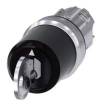
Key-operated switch IKON, 22 mm, round, metal, shiny, lock number 360012K1, with 2 keys, 3 switch positions I-O-II, latching, actuating angle 2x45°, 10:30h/12h/13:30h, Key removal I+O+II, with laser labeling, upper case and lower case, always upper case at the beginning of the word
