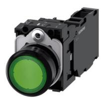
Illuminated pushbutton, 22 mm, round, plastic, green, pushbutton, flat, momentary contact type, with holder, 1 NO+1 NC, LED module with integrated LED 24 V AC/DC, screw terminal, Z=20-unit packaging
