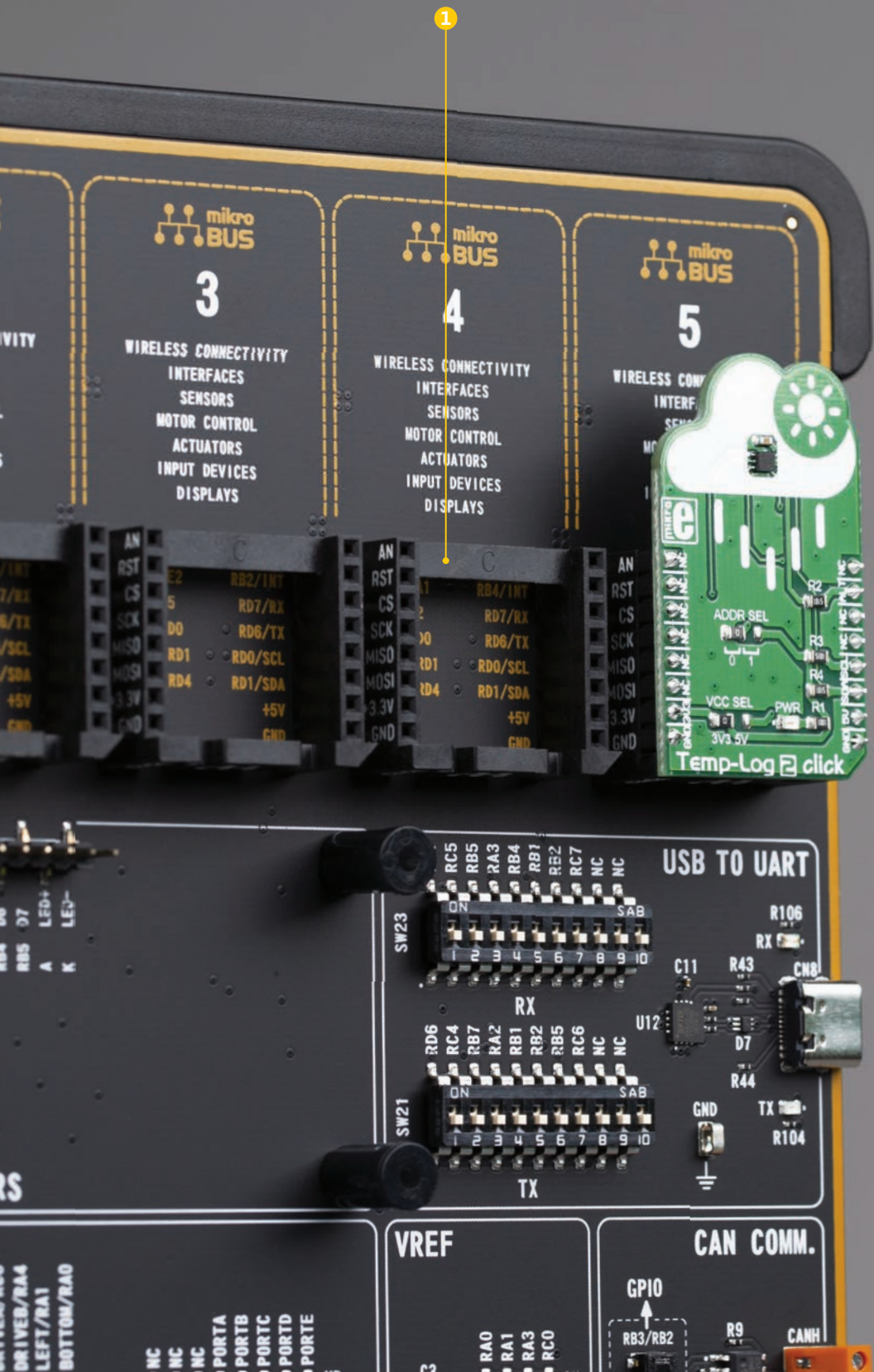
Figure 12: Main board with mikroBUS™ socket close up view
