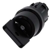
Key-operated switch O.M.R, 22 mm, round, plastic, lock number 73034, black, with 2 keys, 2 switch positions O-I, latching, actuating angle  $90^\circ$ , 10:30h/13:30h, key removal I, with laser labeling, upper case
