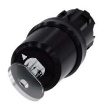
key-operated switch Siemens, 22 mm, round, plastic, lock no. LSG1, with 2 keys, 2 switch positions O-I, latching, actuating angle  $90^\circ$ , 10:30h/13:30h, key removal O, with laser labeling, upper case and lower case, always upper case at the beginning of the word
