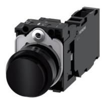
Pushbutton, 22 mm, round, plastic, black, pushbutton, raised, momentary contact type, with holder 1 NO+1 NC, screw terminal, with laser labeling, inscription or symbol Customer-specific selection with SIRIUS ACT configurator (CIN)
