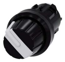
Selector switch, 22 mm, round, plastic, white, Rotary knob, 4 switch positions I-II-III-IV, latching, Actuating angle 4x90°, 3h/6h/9h/12h, with laser labeling, upper case and lower case, always upper case at beginning of line
