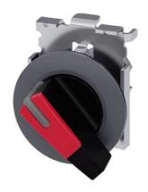
Selector switch, illuminable, 30 mm, round, Metal, matte, red, selector switch, long, front ring for flush installation, 2 switch positions O<I, momentary contact type, Actuating angle 45°, 10:30h/12h, with laser labeling, lower case
