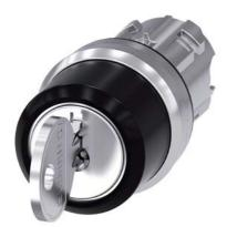
RONIS key-operated switch, 22 mm, round, metal, shiny, lock number SB30, with 2 keys, 3 switch positions I-O-II, latching, actuating angle 2x45°, 10:30h/12h/13:30h, Key removal II, possible special locks: SB31, 421, 455, with laser labeling, upper case
