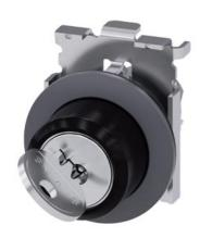
RONIS key-operated switch, 30 mm, round, Metal, matte, front ring for flush installation, special lock, with 2 keys, 2 switch positions O-I, latching, actuating angle 90°, 10:30h/13:30h, key removal I, possible special locks: SB31, 421, 455
