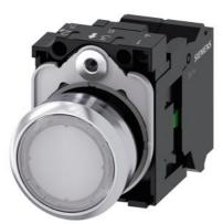
Illuminated pushbutton, 22 mm, round, metal, shiny, white, pushbutton, flat, momentary contact type, with holder, 1NO, LED module with integrated LED 110 V AC, spring-type terminal, Z=20-unit packaging
