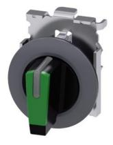
Selector switch, illuminable, 30 mm, round, Metal, matte, green, selector switch, short, front ring for flush installation, 3 switch positions I>O<II, momentary contact type, actuating angle 2x45°, 10:30h/12h/13:30h, with laser labeling, inscription or symbol Customer-specific selection with SIRIUS ACT configurator (CIN)
