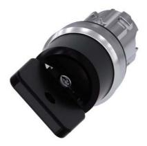
Key-operated switch O.M.R, 22 mm, round, metal, shiny, lock number 73034, black, with 2 keys, 2 switch positions O-I, latching, actuating angle 90°, 10:30h/13:30h, key removal O+I, with laser labeling, inscription or symbol Customer-specific selection with SIRIUS ACT configurator (CIN)
