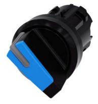
Selector switch, illuminable, 22 mm, round, plastic, blue, selector switch, short, 2 switch positions O-I, latching, actuating angle 90°, 10:30h/13:30h, with laser labeling, inscription or symbol Customer-specific selection with SIRIUS ACT configurator (CIN)
