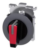
Selector switch, illuminable, 30 mm, round, Metal, matte, red, selector switch, short, front ring for flush installation, 3 switch positions I-O-II, latching, actuating angle 2x45°, 10:30h/12h/13:30h, with laser labeling, upper case and lower case, always upper case at beginning of line
