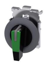
Selector switch, illuminable, 30 mm, round, Metal, matte, green, selector switch, long, front ring for flush installation, 3 switch positions I-O-II, latching, actuating angle 2x45°, 10:30h/12h/13:30h, Z=50-unit packaging
