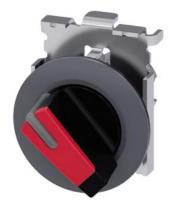
Selector switch, illuminable, 30 mm, round, Metal, matte, red, selector switch, short, front ring for flush installation, 2 switch positions O<I, momentary contact type, Actuating angle 45°, 10:30h/12h, with laser labeling, upper case and lower case, always upper case at beginning of line
