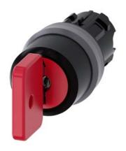
Key-operated switch O.M.R, 22 mm, round, plastic with metal front ring, lock number 73037, red, with 2 keys, 3 switch positions I>O<II, momentary contact type, actuating angle 2x45°, 10:30h/12h/13:30h, key removal O, with laser labeling, lower case
