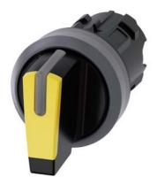
Selector switch, illuminable, 22 mm, round, plastic with metal front ring, yellow, selector switch, short, 3 switch positions I-O<II, left latching, right momentary contact type, actuating angle  $2x45^{\circ}$ , 10:30h/12h/13:30h, with laser labeling, upper case and lower case, always upper case at beginning of line
